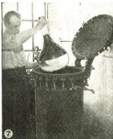
Fig. 7—The Du Mont television tubes are tested at high pressure in compressed air tanks. 8—The finished 14" cathode ray image tube in a receiver.
