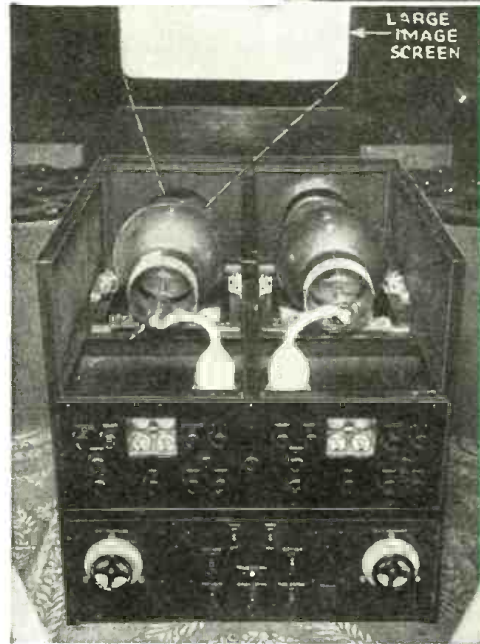
Below—Interior view of the theater television projector, showing the control switch-board and the high voltage cathode-ray tubes. (One is a spare.)
