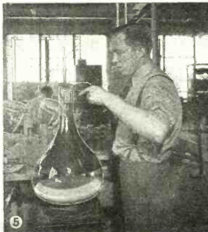
Fig. 5 shows glass expert fusing electron "gun" unit into position. 6—Heating internal metal units with high frequency currents.
