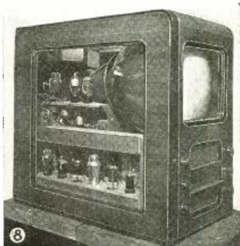
Fig. 7—The Du Mont television tubes are tested at high pressure in compressed air tanks. 8—The finished 14" cathode ray image tube in a receiver.
